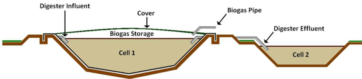
Figure 2 - Covered lagoon schematic. Graphic courtesy of US EPA AgSTAR Program.
